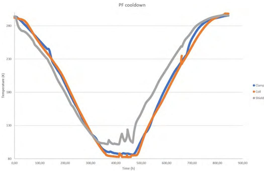
Figure 4 Cooldown and warm up of PF6.
