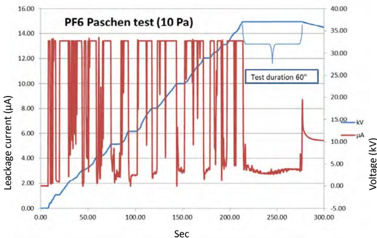
Figure 8 : Paschen tests on PF6.
