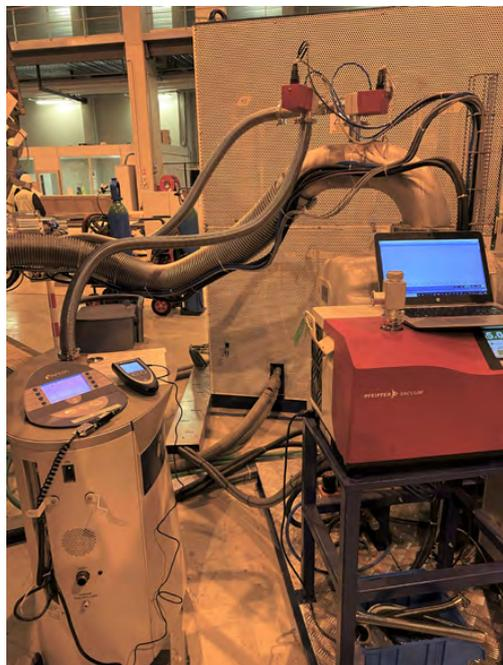
**Figure 6** Leak detector, on left side, and vacuum pumping system connected to PF5 cryostat.
