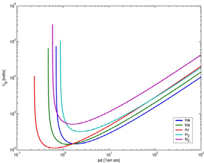
Figure 7 Paschen curves for different gases. He and N2 plots are relevant for the tests on ITER superconducting magnets.
