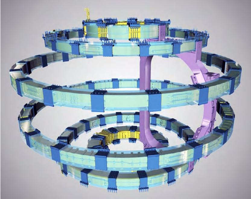
Figure 1 Poloidal field coils of ITER with one toroidal field coil.
